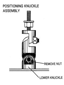
NOTE: PLEASE LOOK OVER THE EXACT MANNER IN WHICH THE POSITIONING ASSEMBLY AND THE ATTACHMENT PLATE GO TOGETHER SO THAT YOU WILL BE ABLE TO REASSEMBLE THEM WHEN YOU HANG THE PROJECTOR.
